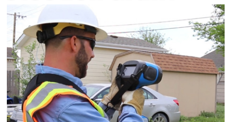
A gas maintenance worker uses laser detection to find a gas leak at the house.
