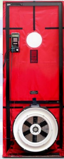
A How$mart audit includes a blower door test which measures air leakage throughout the home.
